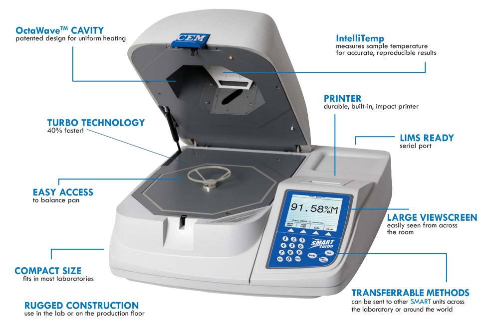
**AOAC-APPROVED METHODS** also complies with other standard methods ACCURATE test precision to 0.01% BUILT-IN MEMORY Stores 100 methods & 300 test results
